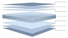
Finish Coat (Finish Coat + Primer = nominal 25µm) {Refer Notes 3 & 4} Universal Corrosion Inhibitive Primer Conversion Coating Zinc-coated steel substrate Conversion Coating Universal Corrosion Inhibitive Primer Backing Coat (Backing Coat + Primer = nominal 10µm total) {Refer Note 5}
